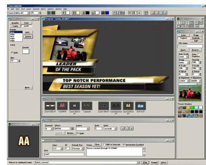
The Avid Deko 3000 Motion Timeline allows easy animation on text, images, and video clips with linked sound effects. Motion Behaviors can be solitary or they can react with on-screen layers, such as repel, attract, skew, dim, and brighten—without requiring complex key-framing. Effects are content-independent; so they work regardless of character count.
