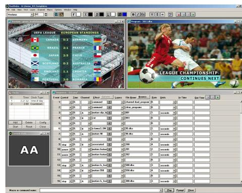
The Avid Deko user interface is designed for core broadcast functions, including manual or automated composition and playback. Avid Deko layers can accept content from a newsroom system, sports interface, or external ODBC database for getting data to air.
